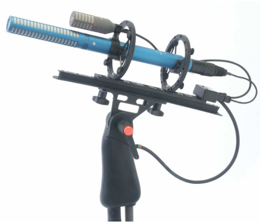
Figure 1: A typical setup for M/S stereophonic recording: shotgun microphone with an attached figure-8 microphone for use in a windscreen. [21]
