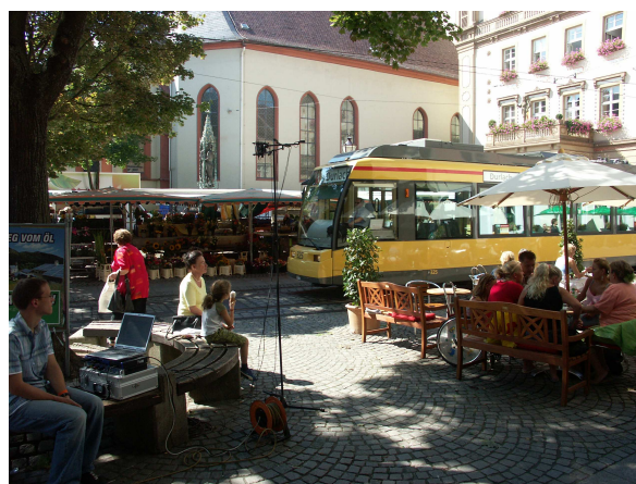
Figure 23: Test recordings using the Double M/S and reference setups: Top picture: Double M/S and OCT surround system in a live theater performance. Bottom picture: Double M/S and an IRT cross setup for an ambience recording at Durlach town square.
