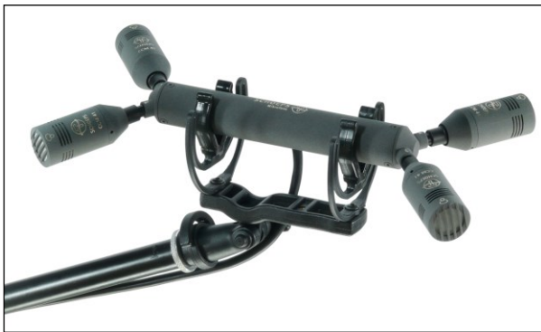
Figure 3: Four-channel “ORTF Surround” system; four supercardioids, 10 / 20 cm spacing, 80° / 100° angles
