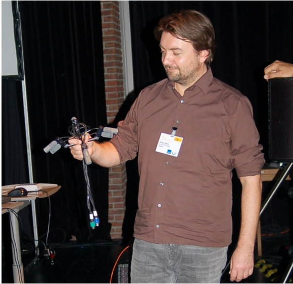
Figure 4: A prototype of the ORTF-3D system at the ICSA conference in 2015. Eight supercardioids, horizontal distance 20 cm, vertical distance 0, angle 90^\circ
