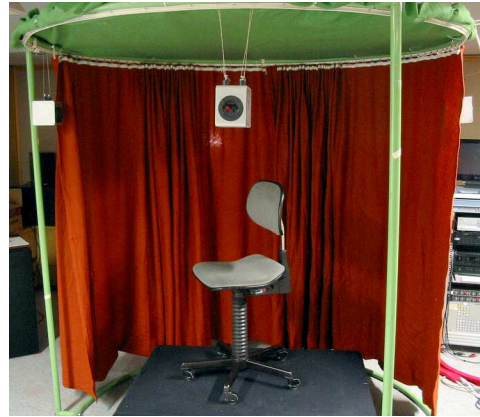
Figure 7: Setup of the localisation experiment with three of the six real sound sources visible. The array is hidden above the horizontal curtain.
